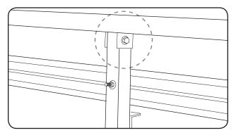
**5.** Center bunks on lift and tighten all bolts.
