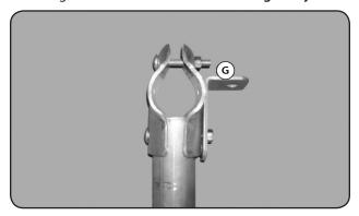
2. Slide the EMPKIT over the Wheel Support Tube (W) in the 6 o'clock position, with the Angle Bracket pointing to the right side of the wheel. Tighten lower bolt first. Then upper bolt.
