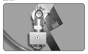
**4.** Slide the Bent Mount Bar (C) through Mounting Bracket (B) with the bent end toward the right side of the wheel. Position with approximately 10" to 11" remaining to the left of Mounting Bracket (B), then tighten the two bolts on the bottom of Mounting Bracket (B).
