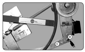
**6.** Rotate the motor up to meet the lift wheel and attach the Spring to the motor as well as the Angle Bracket ((G) in step 1) by using Carabiners provided. **NOTE: Make sure rubber wheel lines up with red wheel on lift.**
